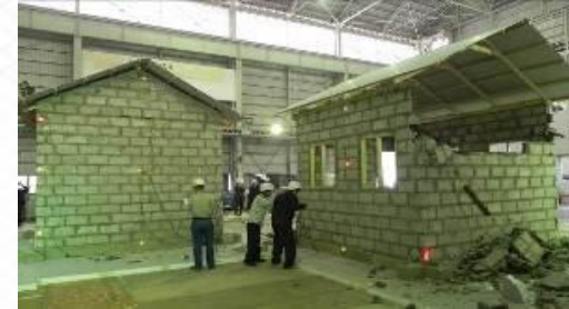
Two full-scale RM (CHB) buildings tested by Imai et al. (2015)
