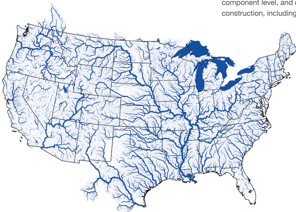
AIR's model captures inland flood risk for 18 hydrological regions across the contiguous U.S., an area of more than 8.2 million square kilometers (3.2 million square miles), with a river network 2.2 million kilometers (1.4 million miles) long represented by over 335,000 distinct drainage catchments.
