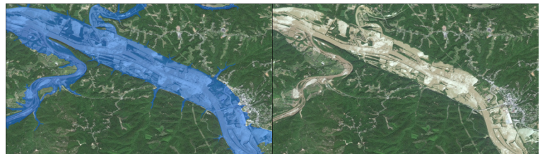
AIR-modeled flood extent (left) and aerial imagery of maximum flood extent from DigitalGlobe (right) near Ashland City, Tennessee, during the 2010 Cumberland River flood.
