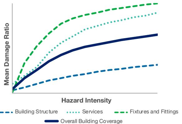
Damage functions for a retail shop in Central Europe show the differences in vulnerability of building components and the combined result for the building overall.
