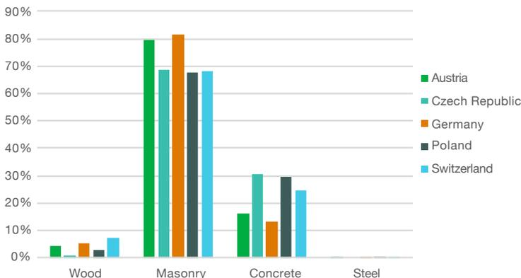
Most residential building stock in Central Europe is of masonry construction, as shown for apartments and single-family homes.
