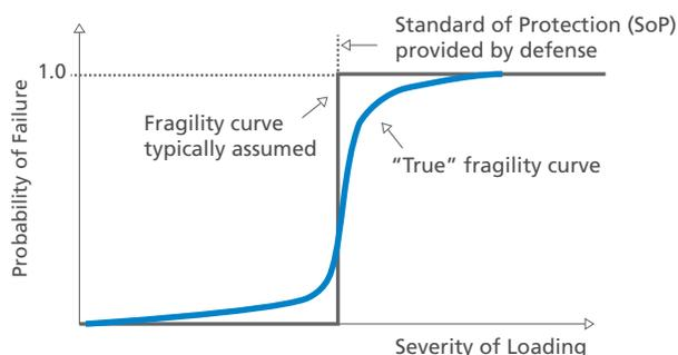
Fragility curves provide the probability of flood defense failure.
