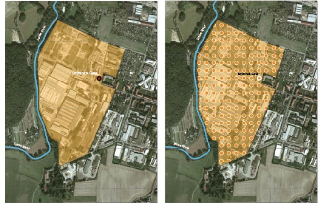
Figure 5. (Left) Total insured replacement value assigned to the main entrance gate of the site. (Right) An exposure grid assuming a uniform distribution of the total insured value over 156 grid points. Modeling this site based on a single geocode (on the left) would severely underestimate the site's loss potential. (Source: Google Earth and AIR)
