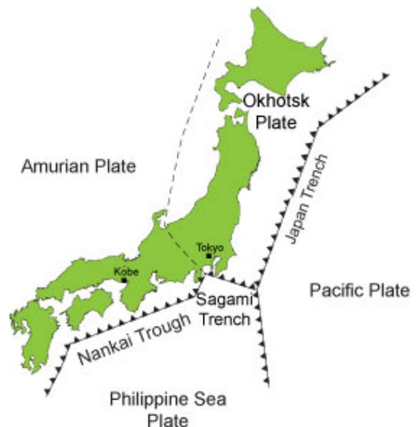
Figure 1: Japan's Tectonic Plates (the arrows show relative motion of the oceanic plates with respect to the continental plates). Source: AIR Worldwide.
