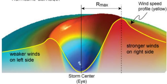
Figure 1. Schematic cross section of a hurricane wind field.  $R_{max}$  is the distance from the center of the storm to the location of the maximum winds. Note how winds are strongest on the right-hand side of the hurricane (assuming a northward direction) due to the additive effect of the hurricane's winds and the storm's forward motion. Source: AIR.
