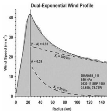
Figure 3. Dual-exponential profile (dark curve) used to approximate the observed wind (shaded). Two distances  $x_1$  and  $x_2$  (dashed curves) control the decay rate of the wind profile outside  $R_{max}$ . (From Willoughby, 2006).
