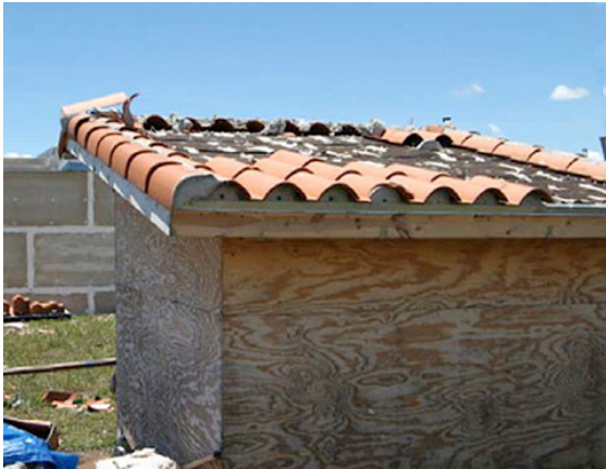
Figure 2. Destructive testing of roof tiles conducted at the Wall of Wind (Source: Huang et. al, courtesy of Wall of Wind, Florida International University)
