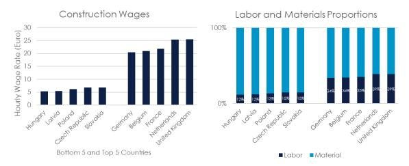
Figure 7. Top 5 and Bottom 5 European countries by construction wage rates (Source: Eurostat, AIR)
